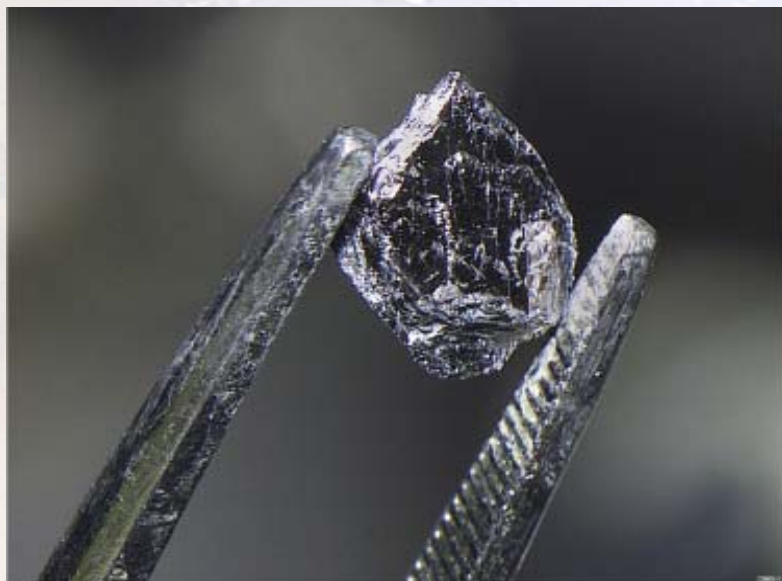
Photographed through a glovebox window, this single crystal of the superconductor plutonium-cobalt-pentagallium was formed using the flux-growth technique.
